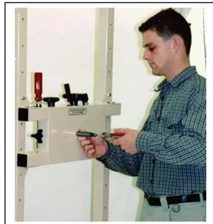
**WC-215 Rotation Activity Module –** Variable-resistance rotation activity for upper extremity exercise. Interchangeable handles and knobs are included. Torque wrench supplied to measure resistance settings.
