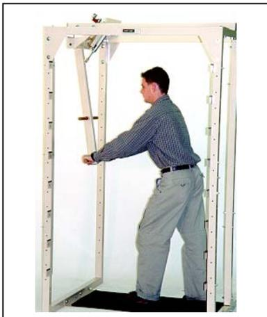
**WC-160 Push-Pull Bar –** Variable-resistance pivot-arm assembly for light-duty pushing or pulling. Similar to weight sled activities.
